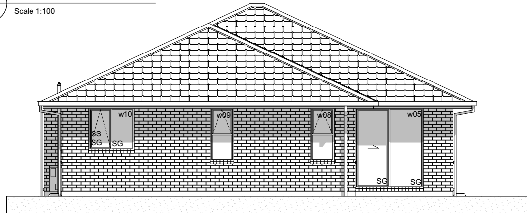
E-03 North Elevation Scale 1:100
