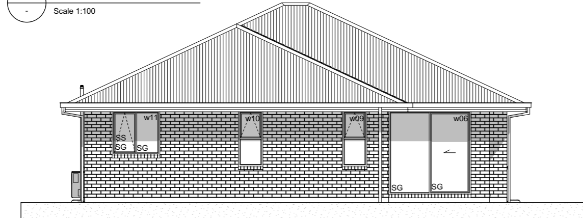
E-03 North Elevation Scale 1:100
